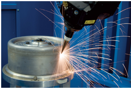
Prima Power Laserdyne specializes in 3-dimensional laser cutting, drilling, and welding.
