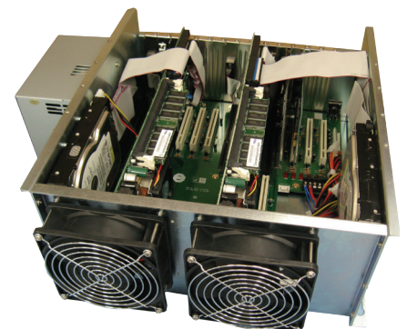
To meet Laserdyne's specific project requirements, CCS designed a custom open frame dual computer system with a long lifecycle in mind.
